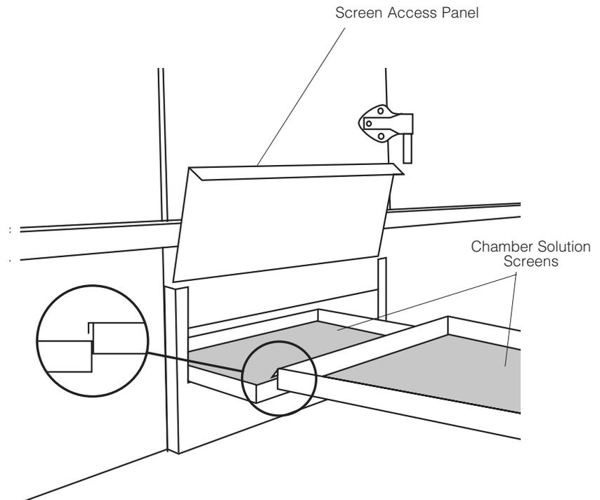
**Figure 6-1. Two-Piece Solution Screen**
