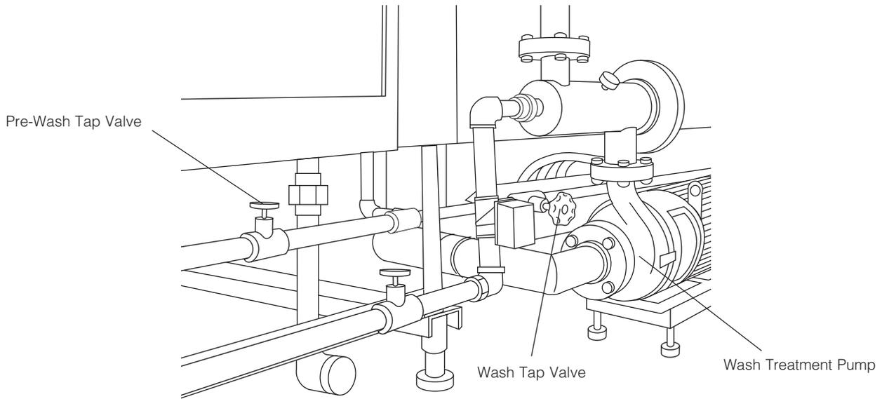
**Figure 6-9. Close Pre-Wash and Wash Tap Valves**
