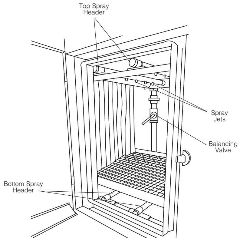
**Figure 6-2. Spray Header Removal**
