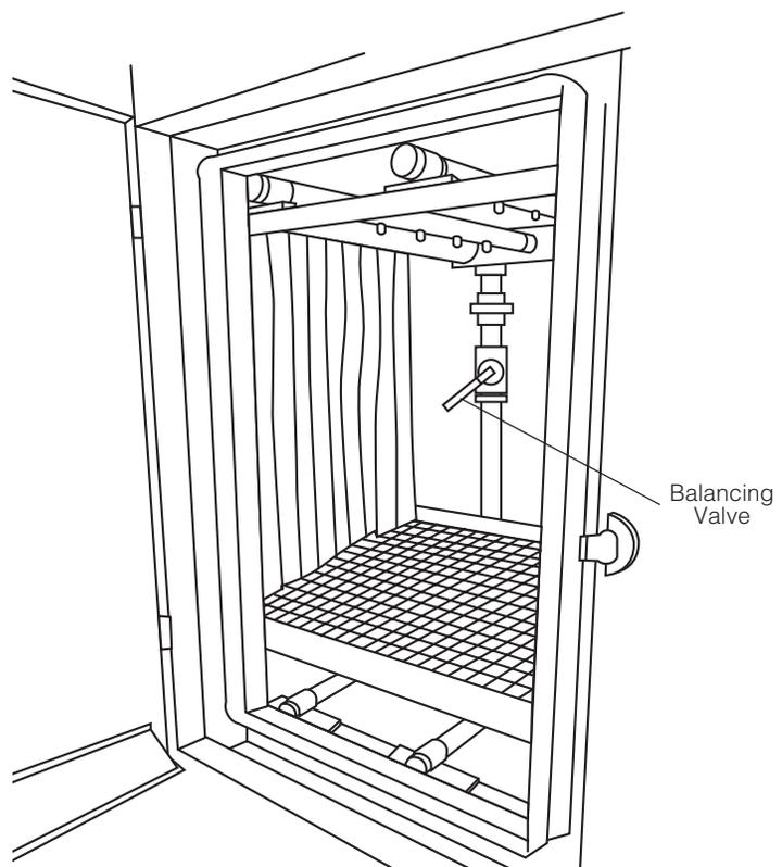
**Figure 6-11. Balancing Valve Location (Typical)**
