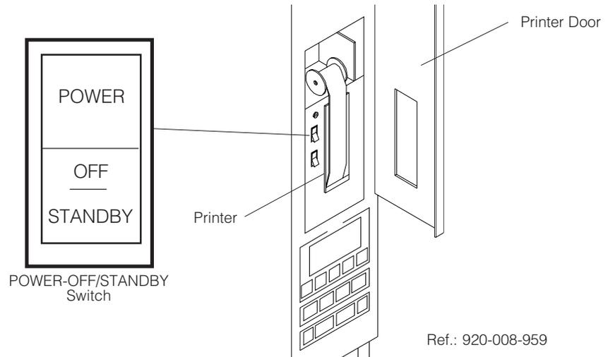
**Figure 3-2. POWER-OFF/STANDBY Switch Location**
