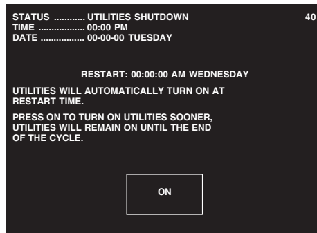
Screen displayed in Auto Utility Shutdown.
